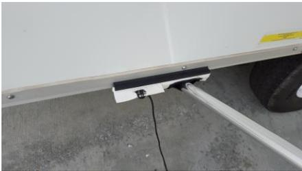
7. Lastly, adjust the tensioners on each guyline so that the Visor is snug and held in place securely by the guy lines. For further instructions on how to use the guy line tensioners, please see the User Tips page (included).
