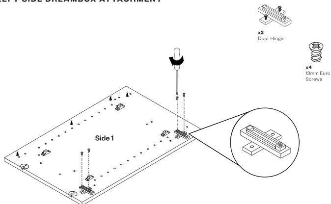
**Note:** Use phillips head screwdriver at a slight angle to tighten built in cams.
