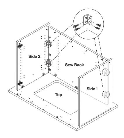
Install **Sewing Base**, tighten cams.
