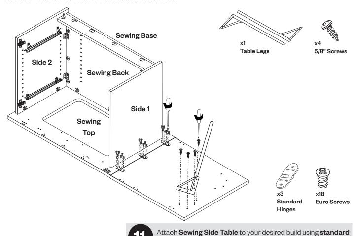
hinges and euro screws. Install table leg with included screws.
