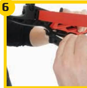
**6.** While holding the 2 nuts in place with your fingers, flip the crossbow over and insert the bolts into the opposite holes. Secure the bolts in place with the correct Allen wrench provided.
