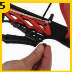
**5.** Drop the 2 nuts into the slots provided on the grip.
