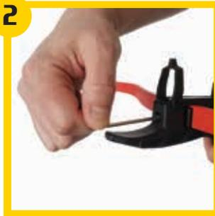
**2.** Tighten retaining screw using the wrench provided. Do not overtighten.
