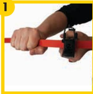
**1.** Back out the retaining screw with the correct Allen wrench provided, until the screw is not visible within the stock opening. Do not unscrew completely. Insert the limb into the stock so that the white lines are even on either side of the stock opening. Place the two rubber pads on the front and back side of the limb within the stock opening. Place the metal pressure pad in between the front rubber pad and the retaining screw.
