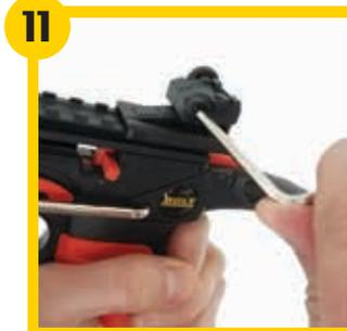
**11.** If the bolt is striking either high or low, use the correct Allen wrench to loosen the bolt on the sight. Adjust the sight to your desired position and then re-tighten bolt to secure.
