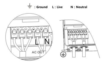
Note: The grounding wire shall be as thick as possible (cross-sectional area is not less than 4mm2). The grounding point shall be as close as possible to the all-in-one solar charge inverter. The shorter the grounding wire, the better.
