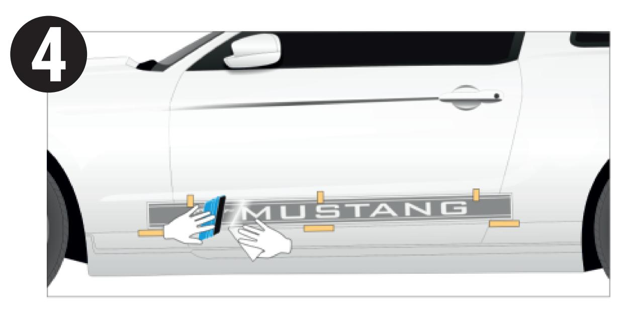
Once aligned, firmly press your hand down the application tape while removing more of the backing at the same time, slowly working your way down the decal. Use the vinyl squeegee to firmly squeegee the application tape, working out any air bubbles from behind the vinyl. The vinyl is now bonding to the vehicles surface.
