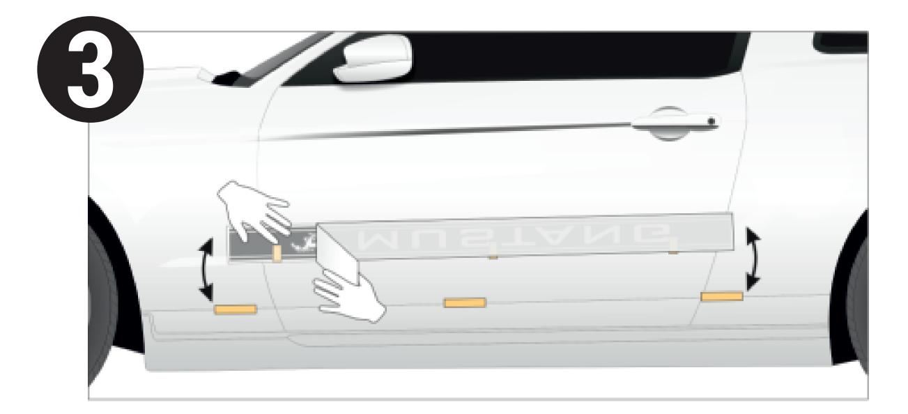
Partially remove the backing from the application tape/decal about 1/4-1/2 way.
