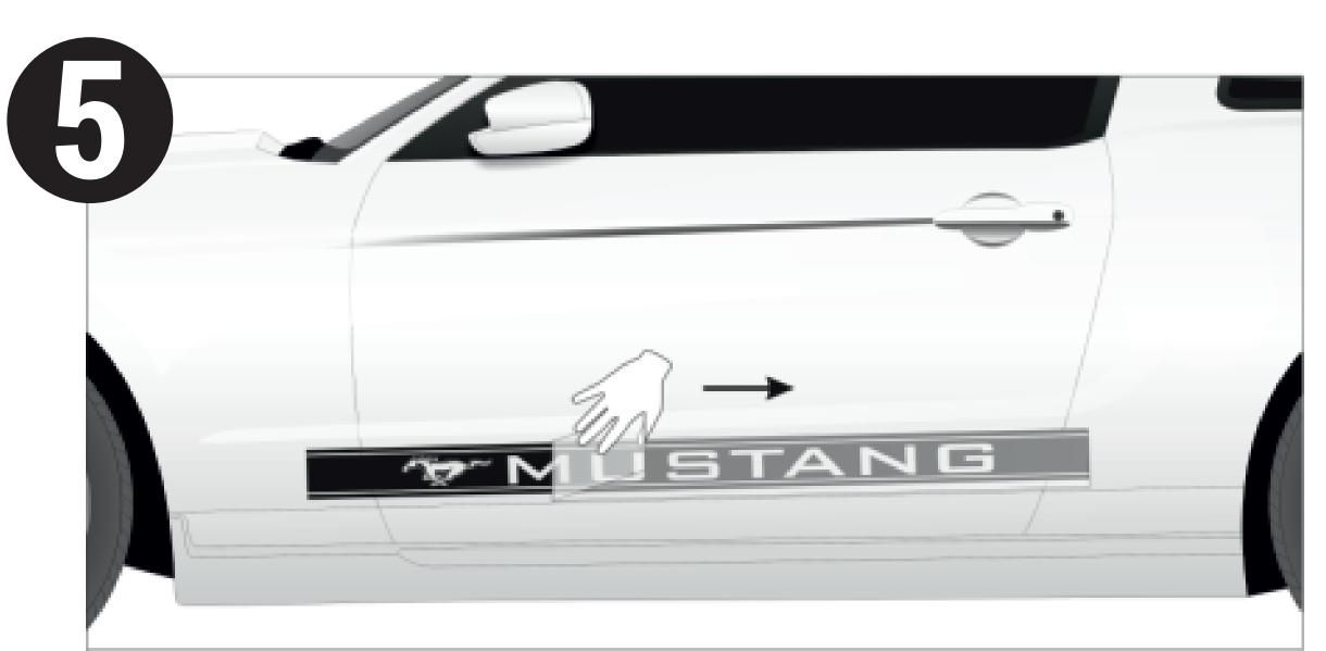
Carefully and slowly remove the application tape, pulling it off at the top corner at a 45 degree angle. If any air bubbles remain, they will usually disappear after a few weeks.
