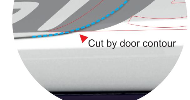
Install second part, remove transfer tape, cut out by door contours, remove cutted part. Cut by door contour
