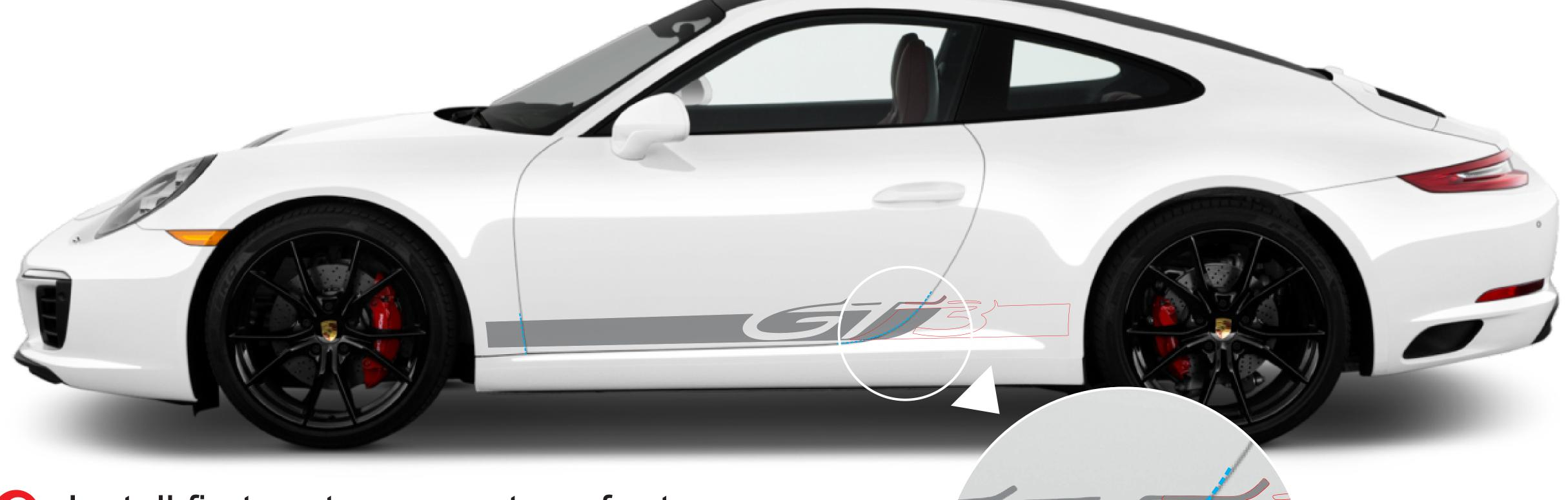
Install first part, remove transfer tape, cut out by door contours, remove cutted part.
