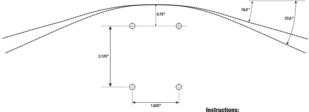
Build your own high performance, low riding longboard. With a good cutting tool (bandsaw, jigsaw, lightsaber, etc), use the included stencil template to trim the nose and tail of your deck (it will almost certainly need it to fit the brackets).
