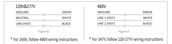
Sensor OR Non-sensor Model Wiring Diagram
