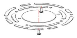
5.Use M4\*25 Self-Tapping screw to fix Support Bracket on the Ceiling.
