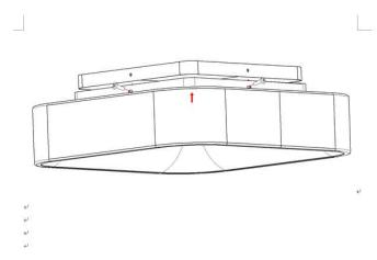
7. Connect wire cable from connector, after finish it, put all the wire connector into J-Box.
