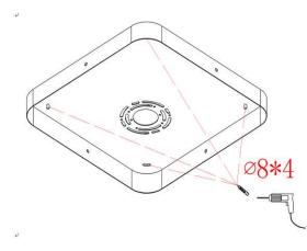
4.Use Screws to fix Support Bracket with J-Box, refer to picture below.
