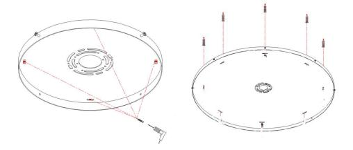
3.Lock M4\*25 Screw with Support Bracket from side, keep the distance from screw head to Support Bracket as 5mm.
