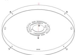
4. Use Screws to fix Support Bracket with J-Box, refer to picture shown below.
