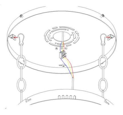
7. Connect wire cable from connector, after finish it, put all the wire connector into J-Box.
