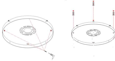
3. Lock M4\*25 Screw with Support Bracket from side, keep the distance from screw head to Support Bracket as 5mm.
