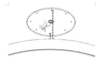
8. Keep the Slot hole as vertical line with Side screw, and make screw into slot, then rotate lamp body, finish fix it.
