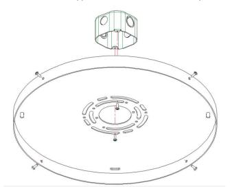
5.Use M4\*25 Self-Tapping screw to fix Support Bracket on the Ceiling.
