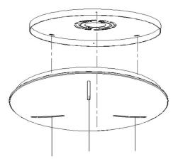
8. After finish installing the ceiling disk, the lamp can be hung. Turn on the electricity, the lamp can be lighted up. After completion of installation, lamp is as following.
