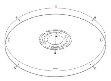
4.Use Screws to fix Support Bracket with J-Box, refer to picture below.
