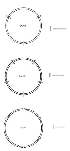
c. Connect the LEDPCB sections Al-PCB wire connection diagram refer to attachment.All Al-pcbs be connected one by one. Following the connection as shown on the picture below.
