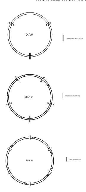
c. Connect the LEDPCB sections Al-PCB wire connection diagram refer to attachment. All Al-pcbs be connected one by one. Following the connection as shown on the picture below.
