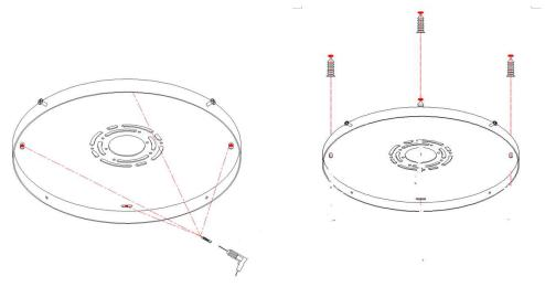
6.Lock M4\*25 Screw with Support Bracket from side, keep the distance from screw head to Support Bracket as 5mm.
