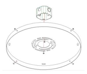
8.Use M4\*25 Self-Tapping screw to fix Support Bracket on the ceiling.
