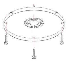
Attention: Must secure mounting plate at all connection points (junction box plus four outer points for small and medium size, or six outer points for large size) to support fixture weight appropriately. Not using all mounting points could damage the fixture and void product warranty.
