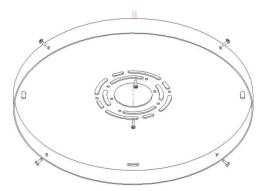
7.Use Screws to fix Support Bracket with J-Box, refer to picture shown below.
