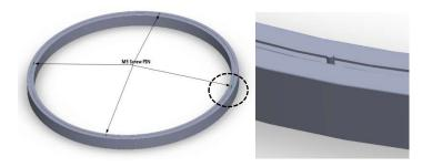
4.Lock the strain relief with M5 hanging pins, see pictures below:
