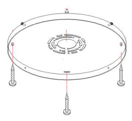
Attention: Must secure mounting plate at all connection points (junction box plus four outer points for small and medium size, or six outer points for large size) to support fixture weight appropriately. Not using all mounting points could damage the fixture and void product warranty.
