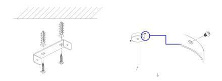
13. Have the two ends of the rope chain insert into the lighting fixture and Fix Pin, Then the ring light is hung! Turn on electricity, ring light will on. Finish installation. See picture below for the installed ring light.
