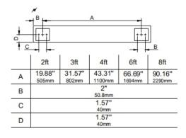
A: Distance between center of two wall boxes B: Distance from center of wall box to the edge of light housing C:Distance between two holes in the wall box D: Distance from center of wall box to bottom of light housing
