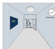
After last detection, the light will be dimmed down to the stand-by dimming level (10%,20%,30% or 50%) after holdtime.
