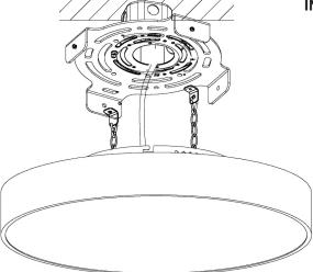
Attention: Must secure mounting plate at all connection points (junction box plus four outer points for small and medium sizes, or six outer points for larger size) to support fixture weight appropriately. Not using all mounting points could damage the fixture and void product warranty.
