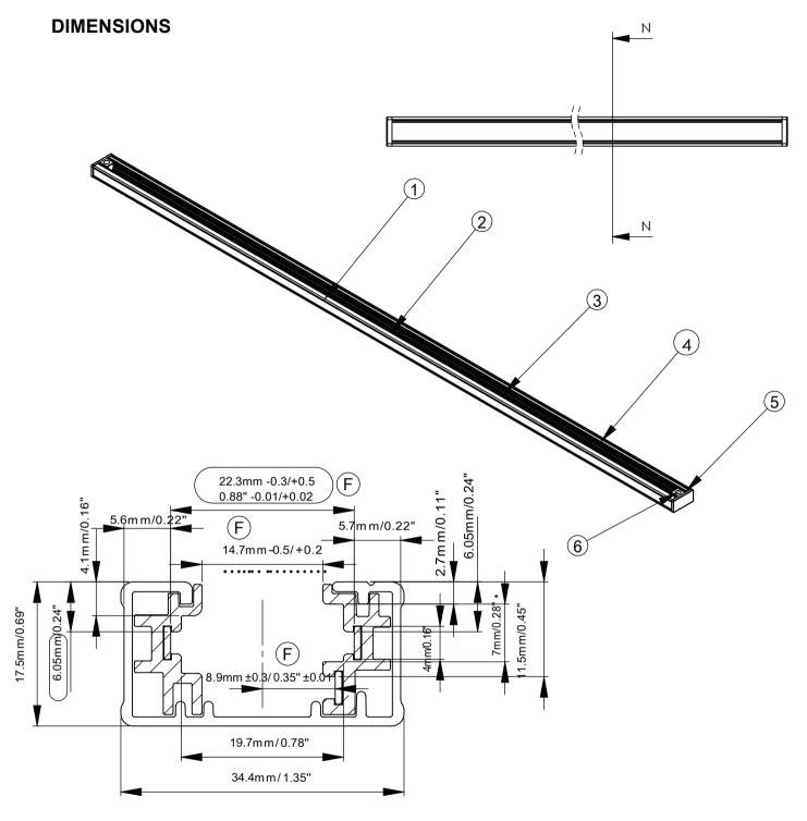
Section: N-N Ratio: 2:1 Length: 4F/47.3"/1200mm 8F/94.5"/2400mm
