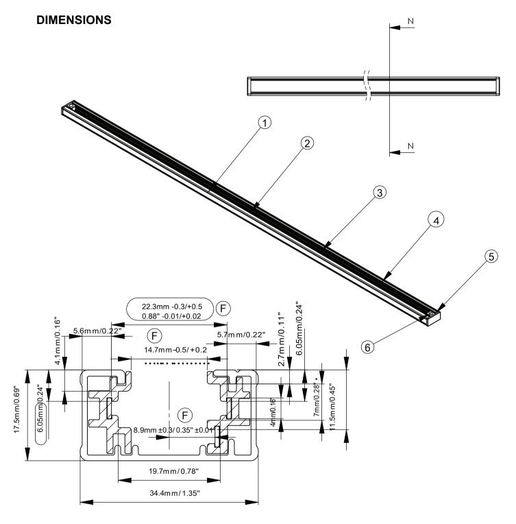
Section: N-N Ratio: 2:1 Length: 4F/47.3"/1200mm 8F/94.5"/2400mm
