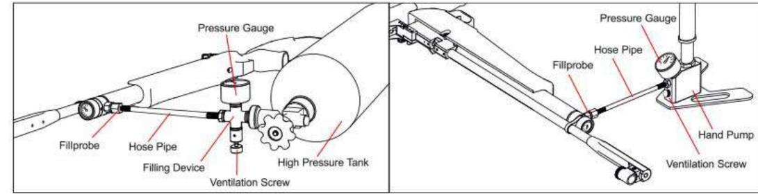
A quick fill connector comes with the rifle and is threaded with a 1/8" BSP male thread to fit the female thread of the hose pipe of the filling device or Hand pump.
