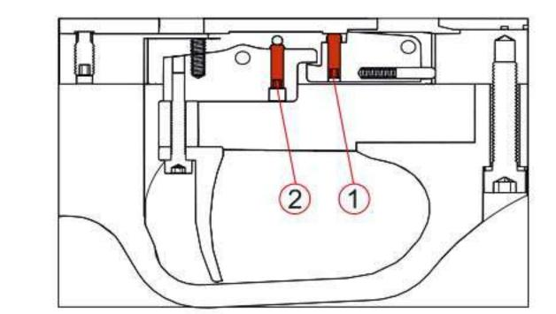
1. Trigger Point / Sear Engagement (Tool required: 1.5 mm Allen Key)
