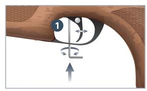
1. Adjustment of trigger take-up (slack): In order to reduce trigger slack: Turn adjustment screw 1 clockwise. In order to increase trigger slack: Turn adjustment screw 1 counterclockwise.
