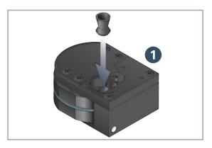
1. Insert the pellet as shown into the pellet chamber of the magazine 1.
