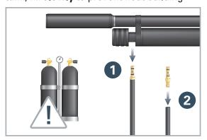
4. Scuba tank: BLEED the fill hose COMPLETELY before disconnecting the quick-fill adapter from the air rifle to avoid hose whip and possible injury. Disconnect the quick-fill adapter from the air rifle 1 and the charging equipment 2. To decock, aim in a safe direction and pull the trigger.
