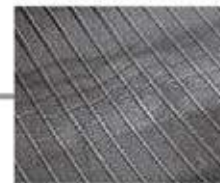
Under-Inflated Tire - An abrasion may run around the circumference of the tire and wrinkles may be observed in the inner liner.
