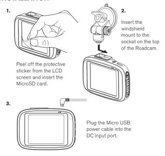
Note: Power on and test camera before mounting.
