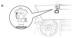
Mount the Roadcam on the windshield. You can turn on the Roadcam and check the live screen to determine the most suitable mounting position. Push the locking lever while pressing the windshield mount onto the glass to secure the camera on the windshield. You are all set!
