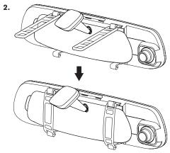
Attach the camera onto your existing rearview mirror using the rubber straps.
