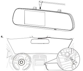
Route the power cable through the headliner and pillars inside your vehicle. Connect the power adapter to your vehicle's 12/24V DC outlet. To ensure it doesn't obstruct the driver while driving, we recommend passing it through the passenger side.
