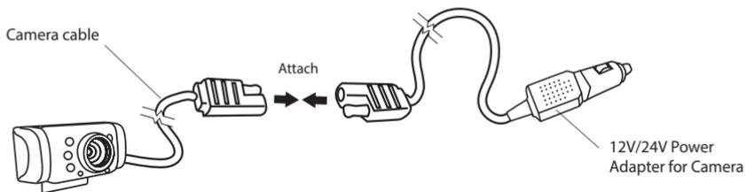
6. Locate the closest available 12/24V socket and plug in the adapter.
