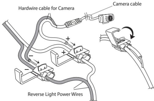
This installation is based on powering the Camera over the reverse tail lights. When installed as directed, the camera image will only appear when the vehicle is in reverse.
