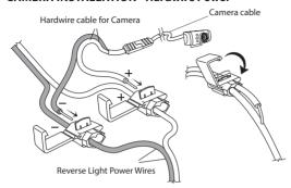
This installation is based on powering the Camera over the reverse tail lights. When installed as directed, the camera image will only appear when the vehicle is in reverse.
