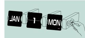
For adjusting the DAY, switch the power to "RAPID DAY" (6), when meets the current day, wait until the current date panel completes and in its position the turn switch to "OFF" (6).
