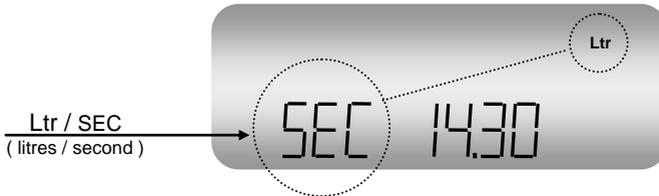
The minimum input frequency for rate display is 0.25hz reducing to 0.1hz If the low frequency cut-off is set to 0.1Hz ( see clause 4.7 ). Rate may be displayed on the large digits on the top display ( see clause 4.8 ).
