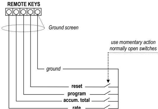
**Wiring requirements :** Use multi-core screened twisted pair instrument cable ( 0.25 – 0.5mm<sup>2</sup> ) for electrical connection between the instrument and any remote flowmeter or receiving instrument. The screen needs to be earthed to the signal ground of the receiving instrument only to protect the transmitted signal from mutual inductive interference.
