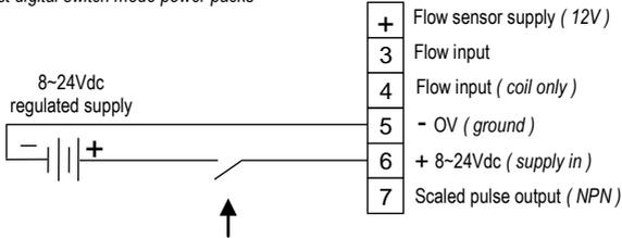
**Note :** Powering the instrument from an external DC source will cause the backlighting feature to turn on, if this is not desirable at all times then install a power isolation switch in series with the DC power source as shown.
