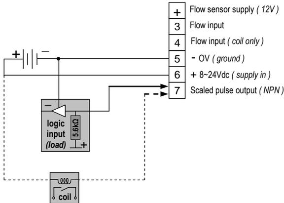
*Driving a logic input* ——— The output voltage pulse is typically the internal voltage of the load. The load would normally have an internal pull up resistor on its input as shown.
