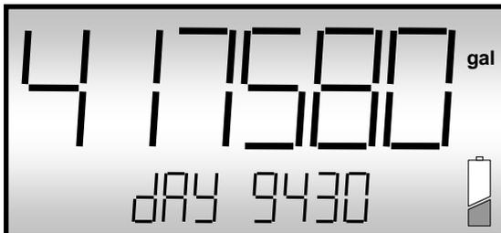
**Backlighting** The LCD backlight feature will only work from an external dc power source in the range of 8~24Vdc.
