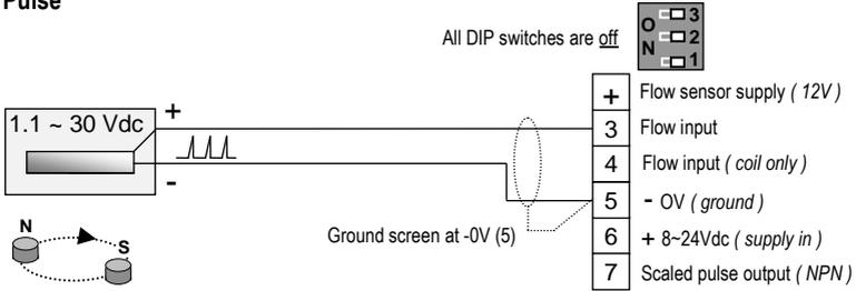
**3. Coil** ( Turbine & paddle style flowmeters – minimum 15mV p-p)
