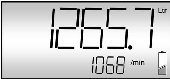
**Rate display** Rate is displayed with a flashing time base of either SEC, /min, /hr or day followed by up to 5 digits of rate; these are programmable for up to 3 "floating" decimal places.
