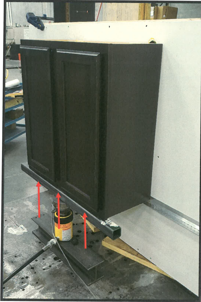
Figure 1: Test setup, cabinet hung upside down for testing purposes, arrow shows load direction.
