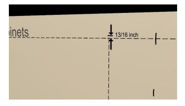
Using your level, extend this line over to where it intersects the closest one of the 2 cabinet layout endpoints.
