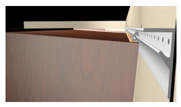
Make sure that the cabinet brackets have engaged the wall rail before releasing the cabinet.
