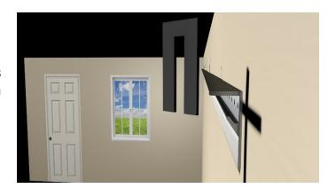
b. Adjusting for high spots in the wall. This is not done now but rather is accomplished when mounting the cabinet brackets. You simply note where on the wall that the high spot is located in the cabinet arrangement, identify the affected cabinet, and then adjust the location of the
