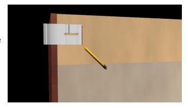
c. Now position the same bracket vertically with the alignment leg resting on the top of the cabinet and transfer the T-nut center mark onto the vertical line. Drill a 5/16" hole through the cabinet from the back. Repeat for the other cabinets.
