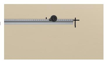
d. Place a level along the top of the wall rail. Adjust the rail until it is level and draw a line along the bottom edge of the rail.
