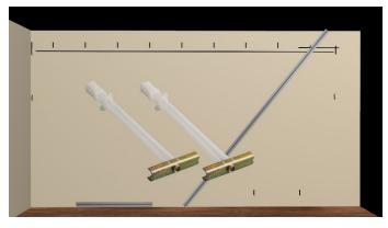
If the end of the wall rail extends 8 inches or less beyond the closest wall stud, then finish attaching the wall rail and the extension using the black oxide 10 x 2" washer head screws at each stud location, making the screws only snug for now.
