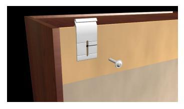
e. With the cabinet mounting bracket alignment leg resting flat against the cabinet top, tighten the screw so that the T-nut barbs engage the face of the cabinet interior rear surface. Repeat for the other cabinets. If you plan to use the decorative plastic T-nut covers, you can install them at this point.
