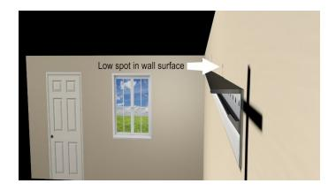
Loosen the rail attachment screws in these low areas and insert the provided plastic horseshoe style shims between the rail and the wall at the stud locations as needed to align the top of the rail in a straight manner. After shims have been added, all of the rail mounting screws should be tightened securely. Re-check the wall rail for straightness and levelness.
