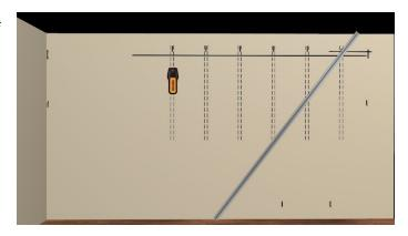
e. With the stud centers located, re-align the wall rail bottom edge on the level horizontal line just made and install another black oxide  $10 \times 2''$  washer head screw in a stud near the center of the rail and another screw in a stud near the end not yet attached, again making the screws snug but not tight.
