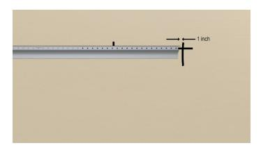
c. Install a black oxide 10 x 2" washer head screw through the wall rail hole into the wall stud whose centerline was just located. Tighten the screw so that the rail is snug but is able to pivot freely. Remove the nail or screw installed as a temporary support from the center of the layout space.
