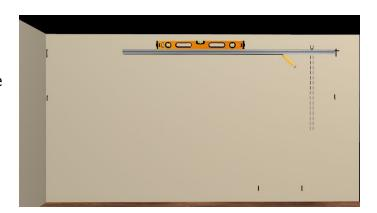
Let the wall rail pivot downward to a resting point while locating the centers of the rest of the wall studs along the line just drawn.
