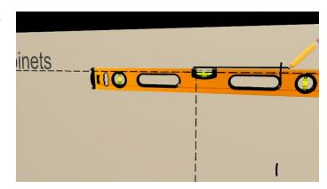
d. Along the horizontal line just made, locate the wall stud closest to the same cabinet layout endpoint and mark this stud's centerline.
