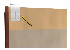
Note: If you have a corner cabinet that attaches to adjacent walls, mark for and install the brackets as shown at locations marked A.
