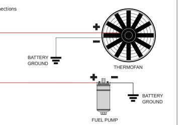
transbrake solenoids, nitrous solenoids etc.
