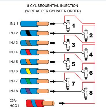
Example wiring connection shown: Sequential injection wiring with 25A-HC01 used as injector 12V. Ensure the high current output used to power the injectors is capable of supplying the required current.
