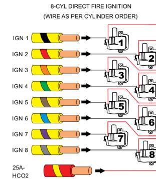
Example wiring connection shown: Direct fire ignition wiring with 25A-HCO2 used as ignition coil 12V. Ensure the high current output used to power the ignition coils is capable of supplying the required current.
