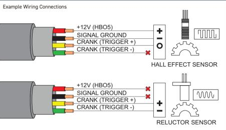
There are two common types of crank/cam sensor sianals:
