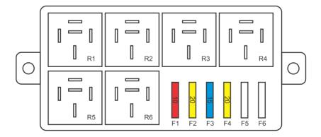
Figure 4 - Haltech Fuse Box Layout
