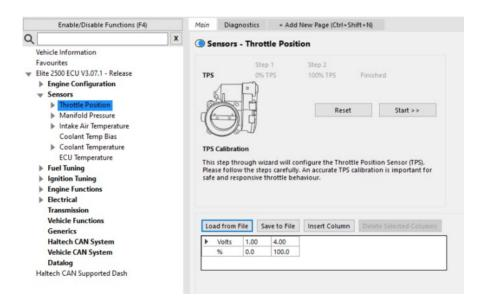
Figure 9 - Throttle Position Sensor Calibration
