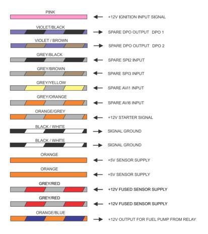
Figure 5 - Cabin Harness Wiring
