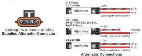
For cases where the alternator uses a different connector, there are optional adapters that can be purchased separately to suit.
