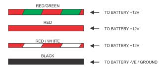
Figure 8 - Battery Wiring
