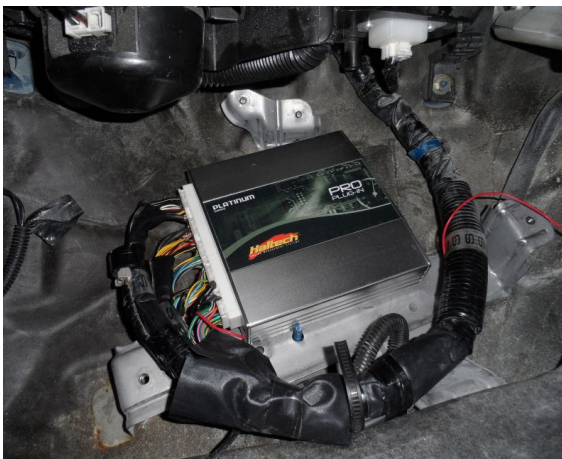
Figure 4 – Haltech ECU Mounted to Factory ECU Mount
