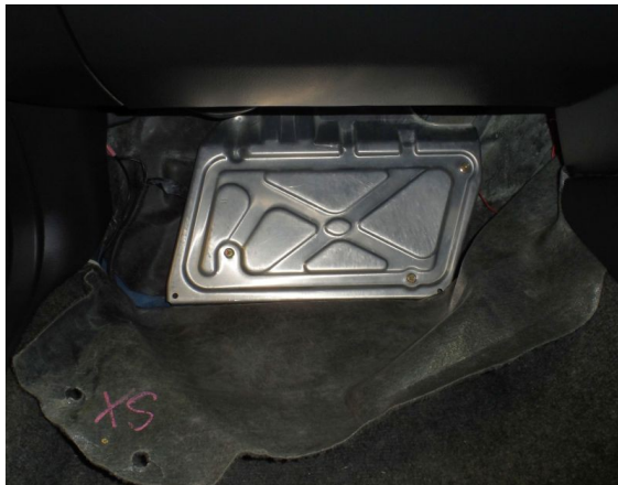
Figure 2 – ECU Protection panel under the carpet
