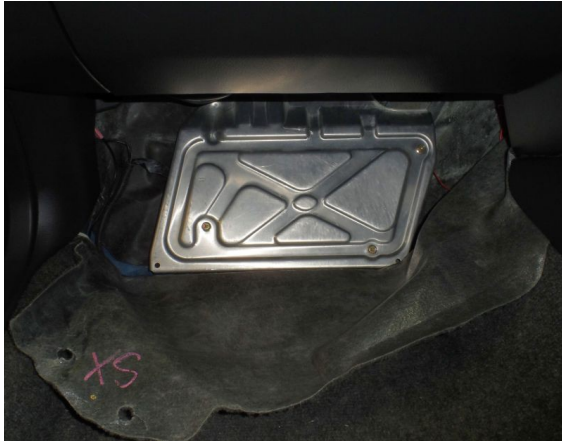
Figure 5 – ECU Protection panel re-installed
