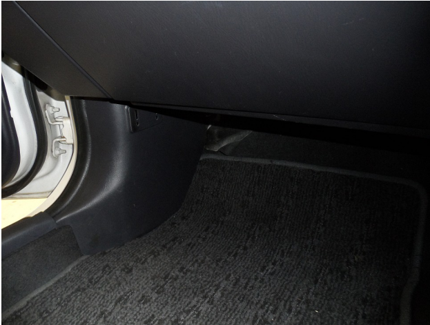
Figure 6 – Kick panel Re-installed
