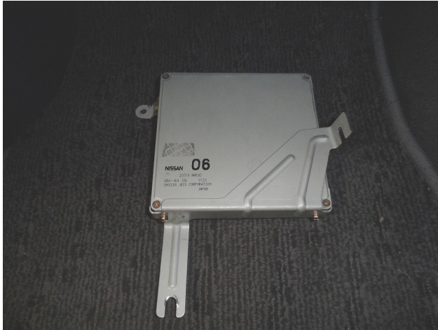
Figure 2 – Factory ECU disconnected and removed
