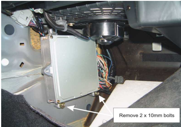
Figure 2 – Factory ECU removal
