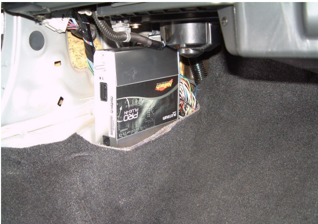
Figure 3 – Haltech ECU Mounted to Factory ECU location
