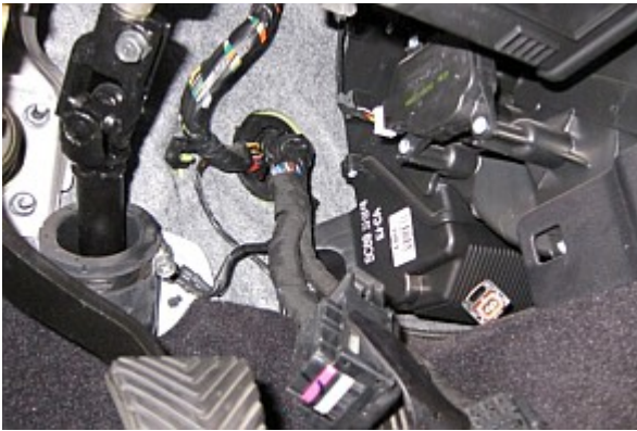
Figure 7 – Factory Wiring Harness Re- Routed into Cabin
