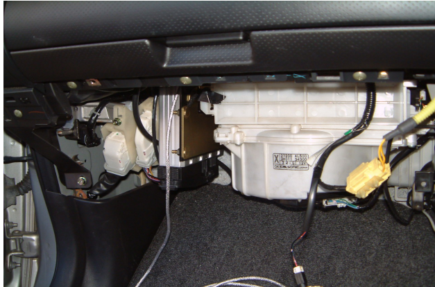
Figure 5 – Haltech ECU Installed in OEM Location
