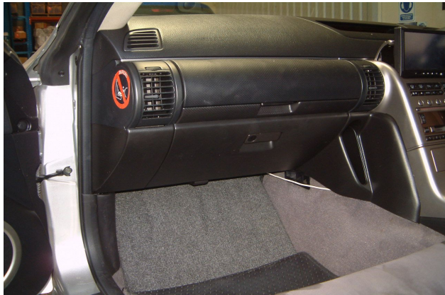
Figure 1 – ECU is located behind the glove compartment
