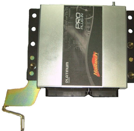
Figure 4 – Platinum Pro Plug-in ECU mounted on OEM mount
