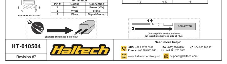
Connect signal to a spare AVI or SPI input on your ECU
