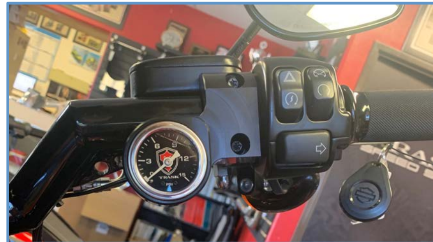
Installed Trask Boost Gauge
