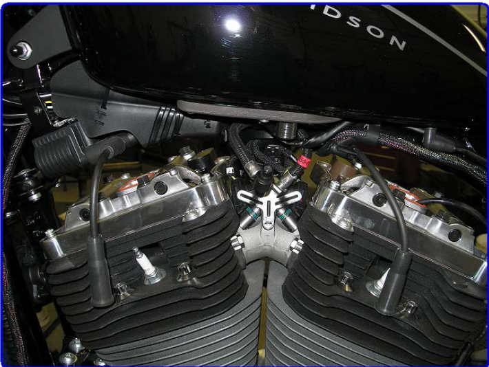
Remove the front and rear rocker box covers.
