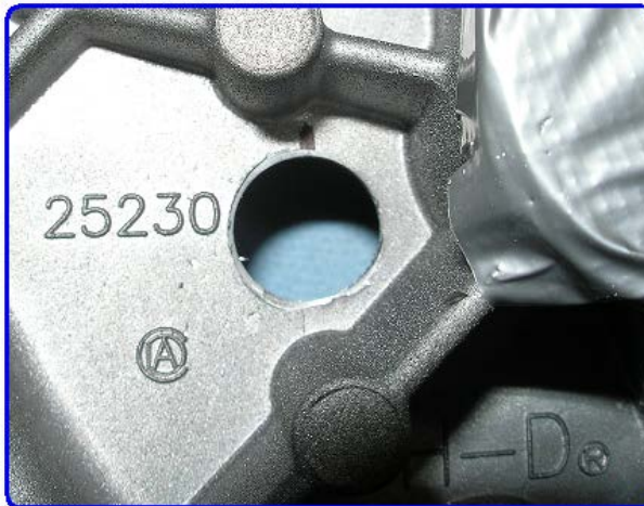
Drilled oil drain hole
