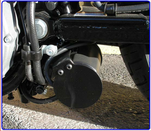
Showing Factory Location of charcoal canister
