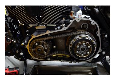
Remove the primary cover. Break loose jam nut and adjust the clutch out. Next remove fasteners for clutch spring as referred to in factory manual.
