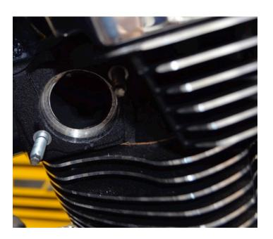
Remove existing exhaust gaskets. Be sure to clean any remaining gasket material prior to installing the new one.
