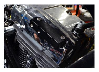
Install the intercooler support bracket onto the front rocker box cover using the supplied hardware.
