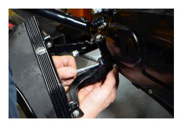
Install the left floor board spacers and torque to spec.
