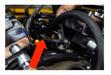
Install the line for the blow off valve on the factory port on the throttle body. NOTE: a black rubber cap will be covering this port on throttle by wire models. On cable models the modification is shown on where to drill and tap for this fitting.
