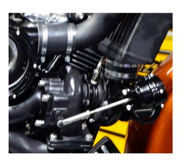
\*\*\*NOTE: When installing the system YOU MUST CHANGE THE OIL. No matter the previous mileage on your last oil change. This reduces particles going through the new turbo. Also fill oil filter ¾ of the way and if possible squirt some in the turbo cartridge prior to tightening the oil feed line. This is crucial to start up as to not starve the turbo of oil.
