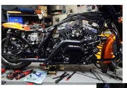
Install the exhaust support bracket at the tranny indicated by the red arrow. Install tail pipe with supplied gasket and loosely thread in fasteners at the exhaust support bracket. Loosely thread in the 5 bolts at the turbo as well. Do not tighten at this time.
