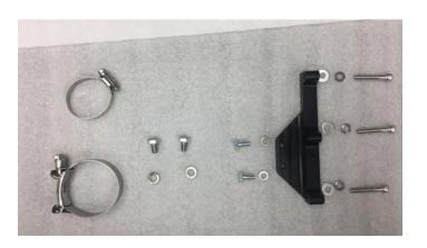
The 02-08 FL models will use this hardware kit. Mounts to the bottom of tranny using the ¼-20 fastenrs.
