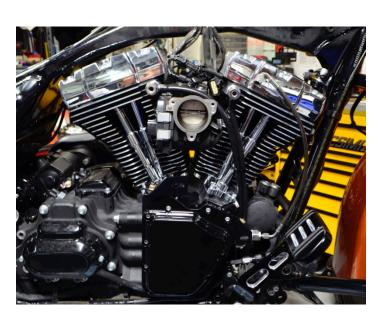
Install the supplied breather bolts and fittings. Torque to spec and route the breathers lines as shown exiting between the frame and motor under the bike. Trim the lines evenly.
