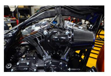
Remove the factory air box. Use the factory service manual for reference.
