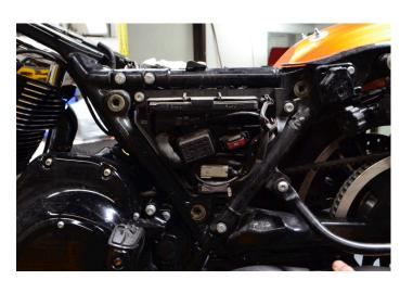
To Disconnect the battery, remove the bags and left side cover. (Remove the "Main Fuse") For your safety and to prevent damage to your bike's electrical system, \*\*\*NOTE: If your bike is equipped with the factory security system it is important that you turn on the ignition BEFORE you remove the Main Fuse. This deactivates your alarm.
