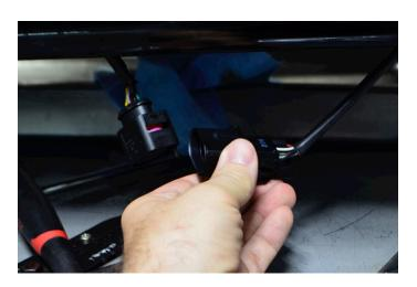
Plug the front o2 into the T-Max harness and zip tie to the frame. Be careful to night make the zip ties too tight.
