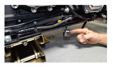
Route the front o2 sensor plug as shown. Use the clips that held the factory o2 harness for the T-Max harness.
