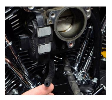
Route the line so it will go on the fitting on the blow off valve.
