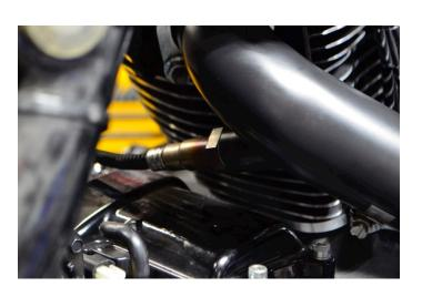
Install the rear o2 sensor and route to plug into the T-Max harness.
