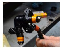
Install the injectors provided in the kit. Depending on year and model you may have to use the adapter block and harnesses. Be sure to lube the o-rings on the injectors prior to installation.
