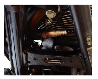
Install the front o2 sensor in the head pipe. Route the harness to meet the connector for the T-Max under the frame.
