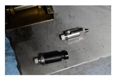
To install the oil feed adapter, locate the oil pressure sending unit and remove. With the supplied pre filter/ oil feed adapter coat the threads with liquid thread sealant.
