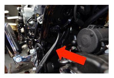
Route the T-Max o2 wire harness through the frame rail as shown.
