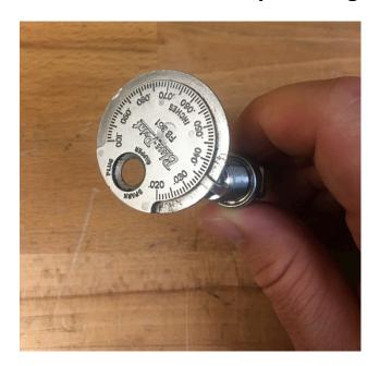
Be sure to gap the supplied plugs to 0.035" and apply copper antisieze to the threads of both plugs and torque to factory specs.
