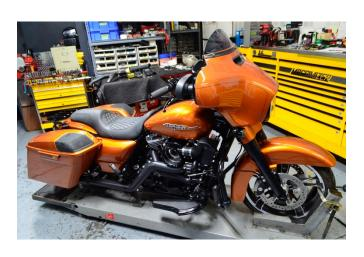
NOTE: Initialize the T-max per Zippers instructions. Start the bike and heat cycle for 2 to 3 minutes then test ride 5 to 10 miles. Once cooled down check over the fasteners again to make sure they have not loosened up.
