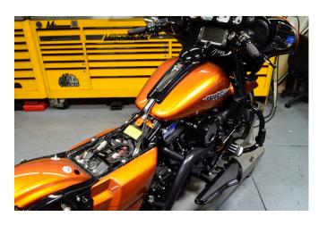
Install the "Main Fuse" along with side covers, bags, tank and seat.
