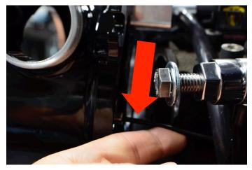
Plug the boost line into the push connect fitting on the back of the plenum.
