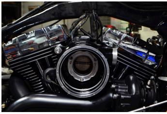
Install and torque the three 1/4-20 SHCS to the throttle body. Tighten the 3/8" hex head and 3/8" SHCS to secure the plenum.
