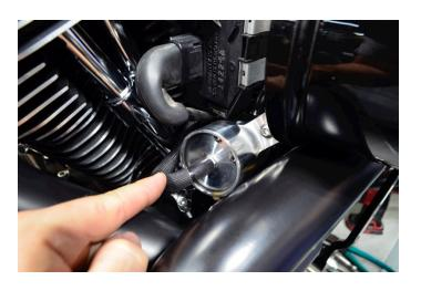
Put the line on the fitting for the blow off valve.
