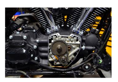
To remove the factory cam cover, remove all fasteners. Be sure to put an oil pan underneath to prevent oil spill. Be sure to clean gasket surface of any gasket material and oil. Remove the brake pedal to gain access to the oil pressure switch.
