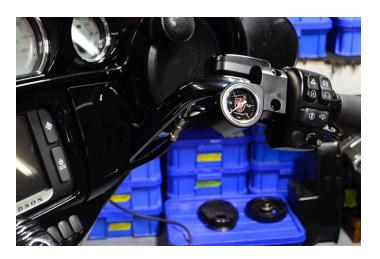
With the boost line in place remove the factory control clamp and replace it with the boost gauge clamp. Torque to spec and insert the line into the push connect fitting then zip tie the line to the bars.
