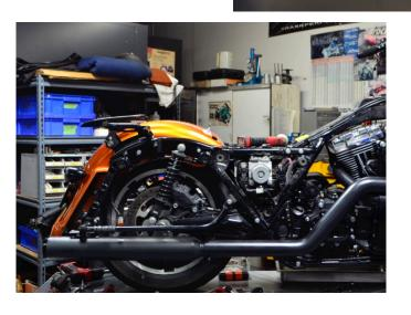
Install muffler. At this time tighten these fasteners in sequence.
