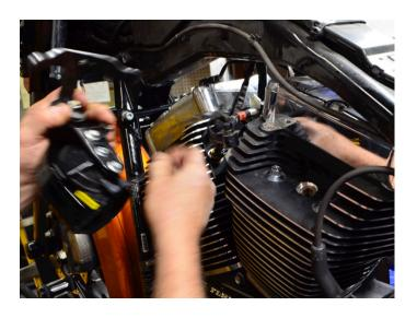
Remove the fastener for the fuel line going into the injectors. To gain access to this remove the horn bracket. Remove the factory injectors.
