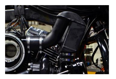
Once the boots are trimmed you can now final install the intercooler tightening the 5/16" SHCS to the support bracket and tighten the clamps in place.
