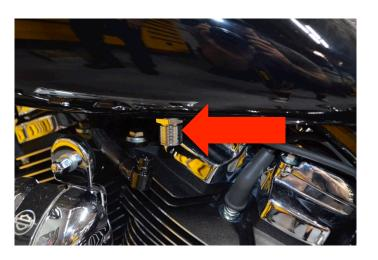
Refer to the Harley service manual for relieving fuel line pressure. This evacuates any built up pressure in the fuel line so you can safely remove the fitting from the tank.
