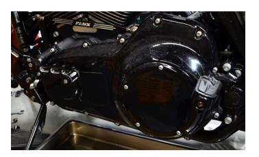
Install primary cover and torque to spec. Reinstall drain plug with new O-ring and thread sealant. Fill primary with oil as per factory spec. You can now adjust the clutch as per Harley spec in the manual.
