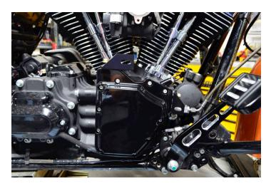
Install the Trask cam cover using the supplied gasket and factory fasteners. Apply blue Loctite and torque to factory specs. \*\*\*NOTE: Orientate header support brackets as shown and DO NOT tighten at this point.
