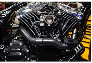
Install the heat shields at this time. Rear first, then the middle with it overlapping the rear shield at the slip-fit. Put the clips, flanges just as you removed from the factory head pipe. Install on the heads. DO NOT TIGHTEN DOWN.
