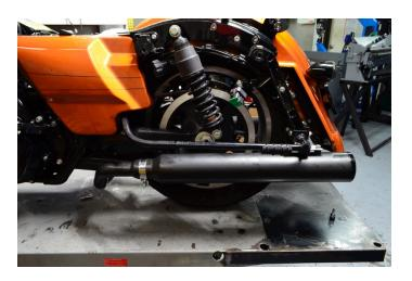
Install the left side muffler and heat shield.
