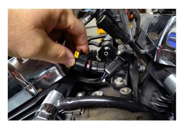
Unplug the factory map sensor. This will plug into the MAP senor on the Trask plenum. For cable bike models a supplied jumper harness will be used to connect the MAP sensor.
