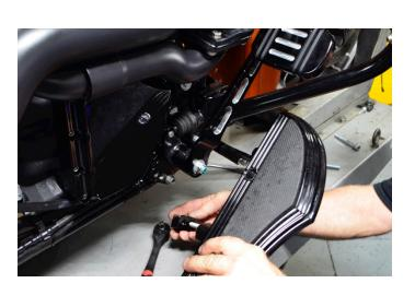
Install right floor board spacers provided in the kit and torque to spec.
