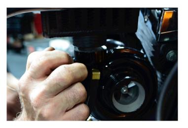
Mock up the intercooler on the rocker box mount to ensure proper orientation of the compressor housing and to trim silicone boots if necessary. Loosen the four flange bolts on the compressor only. Rotate to line the outlet and inlet of the compressor to meet up to the intercooler. Once it is lined up, tighten the four flange bolts on the compressor.
