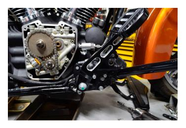
Re-install the brake assembly back onto the frame.
