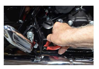
For the other breather line on the right side of the tank, cut the two zip ties fastening it to part of the harness as shown. Pull the line out. Undo the fasteners for the tank and remove the tank.
