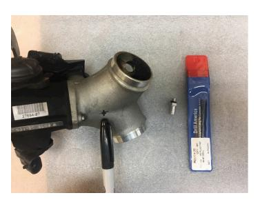
For removal of the 07 and earlier throttle body refer to you Harley service manual. Remove and on the bottom side of the manifold, mark as shown, then drill and tap with the supplied drill and tap (1/4-20). Thread the supplied aluminum fitting with O-ring and be careful not to over tighten. This may cause the fitting to shear off.
