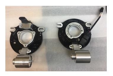
Depending on your model the MAP sensor may require an adapter harness (provided). On the left is throttle by wire which is a direct plug and play. On the right is for cable throttle bodies which requires the adapter harness and will plug into the factory harness.
