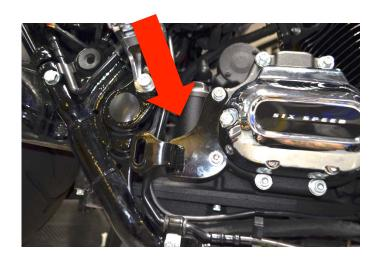
Remove the two factory fasteners on the tranny. Install the supplied exhaust support bracket with washers and fasteners and torque them to factory spec.
