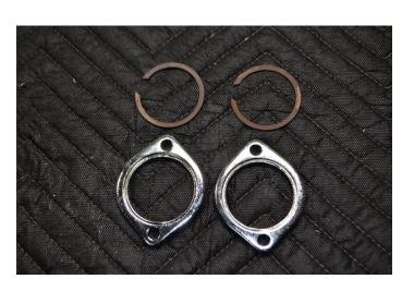
\*\*\*NOTE: DO NOT discard the factory exhaust flanges and retaining clips. You will need these for the turbo head pipe.
