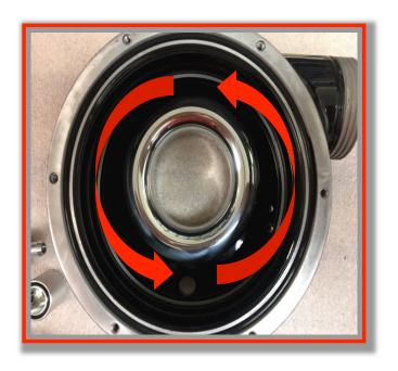
Prior to installing the plenum twist the velocity stack counter clock wise to unlock and pull to remove to access the three holes that mount to the throttle body.
