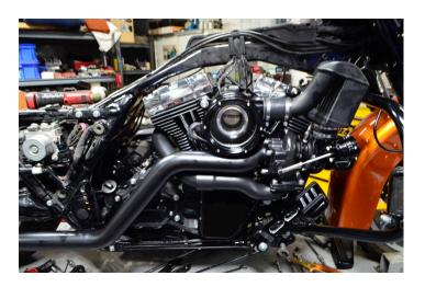
Install the velocity stack, cover and plenum ring.
