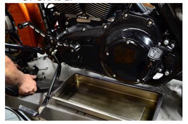
Drain primary oil. While oil is draining collapse the clutch cable. Refer to service manual.
