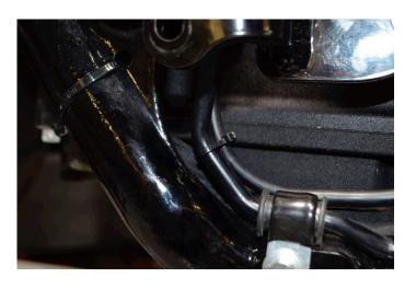
Zip tie and secure the rest of the harness as shown. Do not over tighten the zip ties for o2 wires as the harness has to breath.
