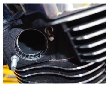
Press the new gasket into the port. Be sure the gasket is seated all the way.
