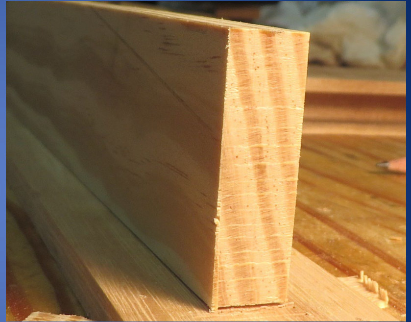
Blonde chisel: end grain is smooth
