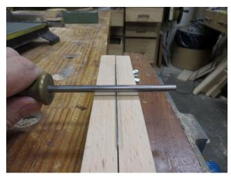
Next, turn the hook by running the burnisher along the edge tilting the burnisher until it is in contact with the edge of the corner of the vise. Tilt the burnisher front to back as you turn the hook so you are drawing the steel out as you push the burnisher along the edge.
