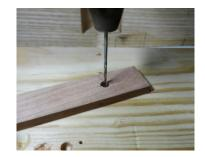
Flip the handle half over and drill the countersink. Drill the countersink just deep enough so the screw head is slightly recessed below the surface. Note: single flute deburring bits are the absolute best at producing the cleanest countersinks with the least chatter.
