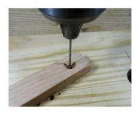
Flip the handle over and use the 1/16" pilot hole as a guide to drill the stepped holes with a 3/8" Forstner bit. Drill the stepped holes slightly deeper than the thickness of the nut. Note: you must use a Forstner bit for this step and not a brad point bit. A Forstner bit will create a flat bottom hole that will not break through the back of the thin blank.
