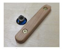
the blank using 220 or 320 grit PSA sandpaper stuck to a piece of plywood. Sand all edges and profiles with 320 grit sandpaper. Carefully separate the halves by inserting a 1/4" chisel in the blade groove and gently twisting to release the double stick tape. Apply a few coats of your favorite finish. Your knife is now ready to put to use.
