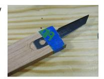
Mark the center of the hole with an awl. Don't worry if your mark is not in the perfect center as the twist drill bit will automatically center itself as it passes through the blade hole. Use a 3/16" twist or machine drill bit and drill the hole with the blade in place. Stop the hole just short of going through the back side. Note: DO NOT attempt to use a brad point or it could catch on the blade and very, very bad things could happen.
