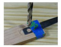
You now need to drill a pilot hole that will guide the countersink bit. Change bits to a 1/16" twist or machine drill bit. Allow the 1/16" bit to fall into the center of the 3/16" hole and drill all the way through the blank. If you hold the blank loosely this will happen all by itself. This 1/16" pilot hole will guide the countersink bit.
