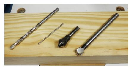
Drill bits needed: 3/16" twist bit, 1/16" twist bit, single flute deburring bit and 3/8" Forstner bit.
