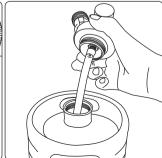
**4.** Install the faucet into the coffee spear and ensure that the connection is proper and tight.
