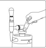
**Note:** It is normal to hear a slight amount of gas escaping and observe a few drops of coffee near the pressure release valve.
