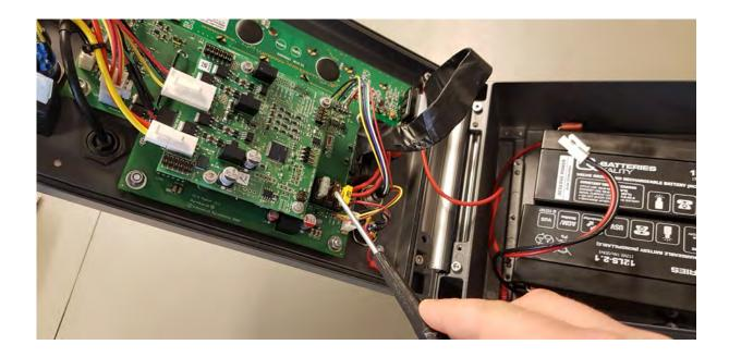
This is the location of the Expansion Fuse. If the fuse is gone, replace it (Mini Blade Fuse 2A 32V slow type). If you are not sure whether the Charger Fuse is gone or not, use a common multimeter to test the fuse for continuity. If you cannot find continuity, the fuse is gone and needs to be replaced.
