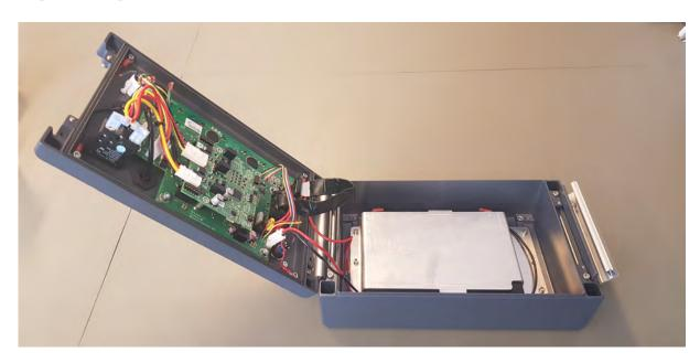
Detach the main fuse. You can easily identify the main fuse by its yellow color.
