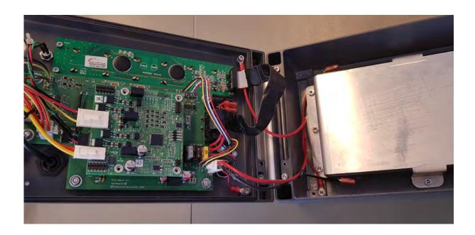
Plug in the Main Fuse before closing the device. Now close the lid. Make sure, that no cables are getting caught and pinched in between the lid and the bottom part of the housing, while closing the lid.
