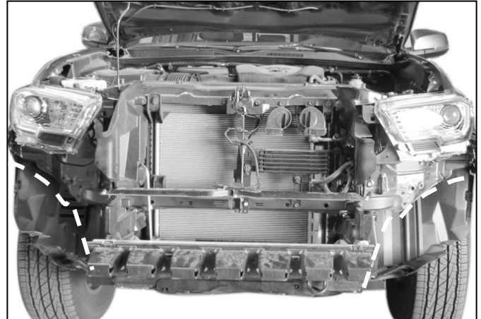
(Fig 9) Remove plastic impact bumper and aluminum crossbar from bumper brackets. Once the Bumper has been installed, trim the plastic covers at the ends as necessary (dashed line)
