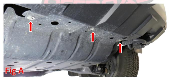
3. Using a 12mm Socket, remove the 5 bolts holding on your skid plate, then remove it. Save two of these bolts. (Fig B)
