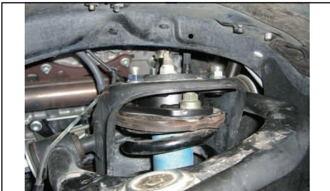
Rotate 180 deg., reattach upper strut with provided hardware
