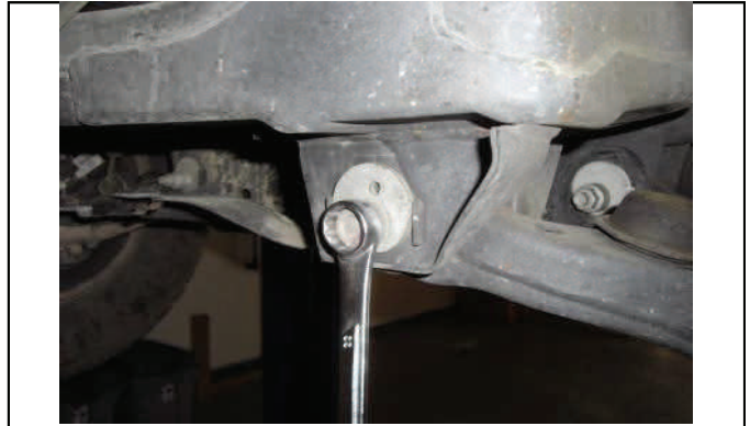
Reset and tighten lower control arm bolts
