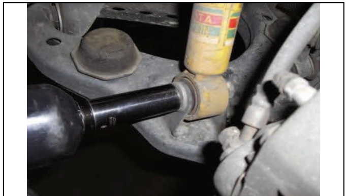
Disconnect lower strut mounting hardware
