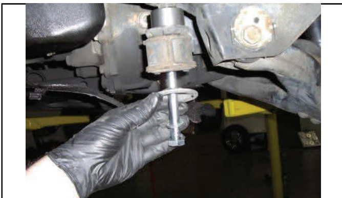
4WD Install longer bolts and reattach differential to frame
