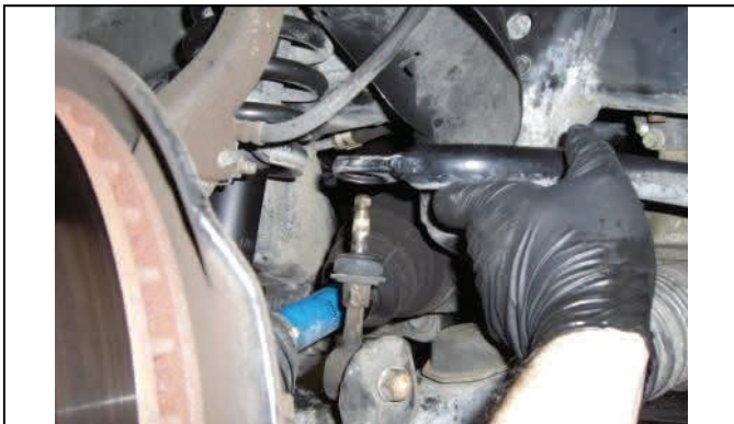
Shows earlier model sway bar end links
