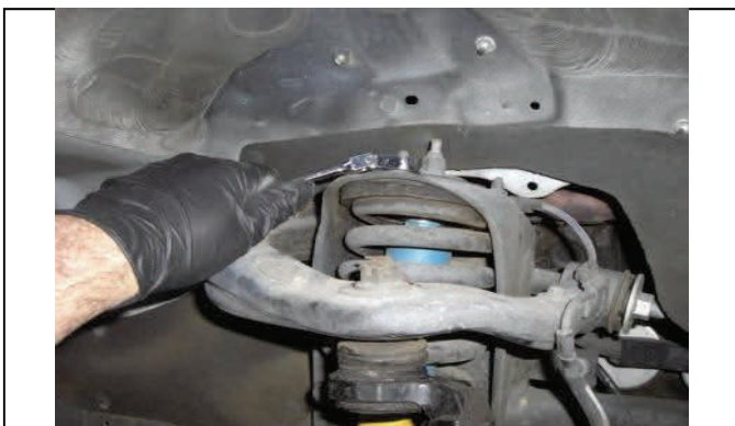
Disconnect upper strut mounting hardware
