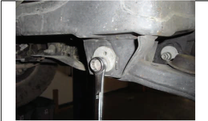
Mark and loosen lower control arm bolts, do not remove
