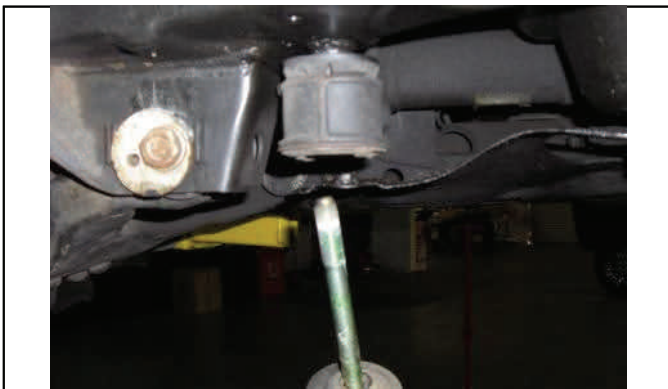
4WD Support differential and remove (2) front mounting bolts
