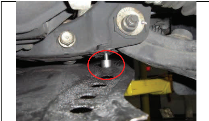
4WD Reattach skid plate with provided spacers and hardware
