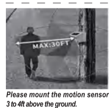
Please mount the motion sensor 3 to 4ft above the ground.
