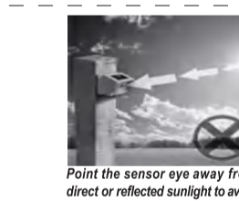
Point the sensor eye away from direct or reflected sunlight to avoid false alarms.
