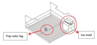
**Ice cube:** The ice cube molds and the tray color tag are gray. Each tray can hold 30 molds and the placement direction is shown as follows:
