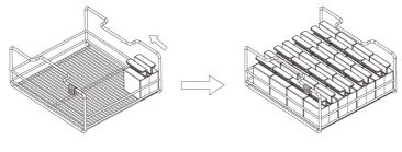
**Ice bar:** The ice bar molds and the tray color tag are black. Each tray can hold 24 molds and the placement direction is shown as follows:
