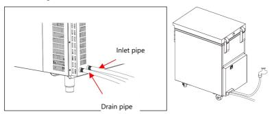
Note: The drain pipe is a corrugated hose about 1 meter long and should be placed into the drainage system. The drain pipe should not be placed higher than the water outlet.
