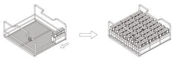
**Ice diamond:** The ice diamond molds and the tray color tag are purple. Each tray can hold 30 molds and the placement direction is shown as follows:
