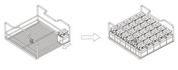
2. Place the tray with the molds on the support blocks in the machine.
