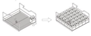
**Ice sphere:** The ice sphere molds and the tray color tag are green. Each tray can hold 16 molds and the placement direction is shown as follows:
