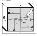
Find the centre of the room using a chalk line, from the middle of wall A to the middle of A1. Then make a line from the middle of wall B to the middle of wall B1. Check that the intersection of the two lines forms a 90° angle.
