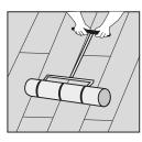
The floor must be rolled with a 50-Kg roller, every 30 minutes, and upon completion of installation, to ensure that the tiles are firmly bedded into the adhesive
