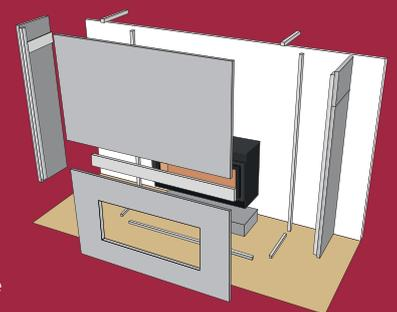
Most enclosures can be built using only Skamol Enclosure, replacing the need for light-frame construction and wall covering. This eliminates a complete stage in the construction process, combining multiple building materials into one.
