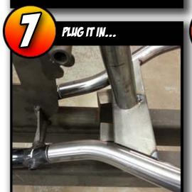
ALTHOUGH WE ARE USING A JIG FOR VISUAL SIMPLICITY, WE RECOMMEND RE-INSTALLING YOUR MOTOR TO ASSURE PROPER FITMENT.
