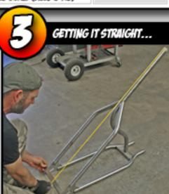
ONCE THE BACKBONE IS IN PLACE OVER THE STUD, TAPE A STRING TO THE TOP CENTER OF THE END. USE A RULER TO ALIGN THE STRING EXACTLY HALF WAY BETWEEN THE AXLE PLATES AND THEN ROTATE THE BACKBONE (LEFT-RIGHT) UNTIL IT BECOMES ALIGNED WITH THE STRING.
