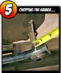
THE FIRST CUTS WILL BE MADE 1" BEHIND THE CENTER LINE OF THE REAR ENGINE MOUNT HOLE. REPEAT ON BOTH SIDES AND CLEAN THE ADJACENT AREA OF THE FRAME TUBES THOROUGHLY!
