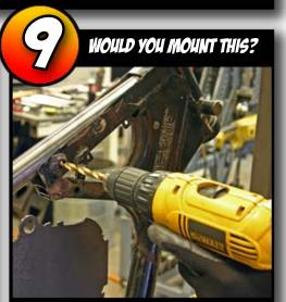
ONCE THE HARD TAIL IS FULLY WELDED IN PLACE, SHOULD YOU WISH TO USE THE TOP ENGINE DAMPER, CAREFULLY DRILL THROUGH THE EXISTING MOUNT HOLE CLEARING THE PATH FOR THE MOUNTING BOLT.
