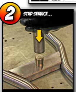
CONTINUE SLIDING AND ROTATING THE BACK-BONE UNTIL IT SLIDES OVER THE 1" STUD AT THE CENTER OF THE CROSS-TUBE. A LITTLE IMAGINATION IS USEFUL, BUT IT WILL WORK!
