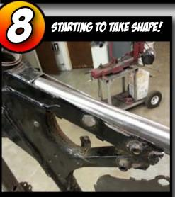
SIMULTANIOUSLY SLIDE THE BOTTOM SLUGS AND THE BACKBONE INTO THEIR RESPECTIVE POSITION MAKING SURE THE TIP OF THE BACKBONE IS TOUCHING THE EDGE OF YOUR CUT LINE. TACK WELD IN PLACE, CHECK ALIGNMENT, THEN APPLY FINAL WELDS THROUGHOUT!
